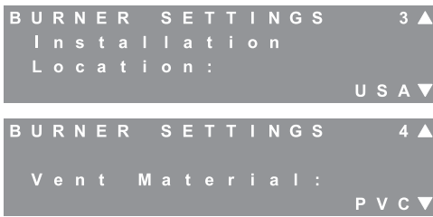
Figure 8.21: Burner Settings – Location & Vent Material
