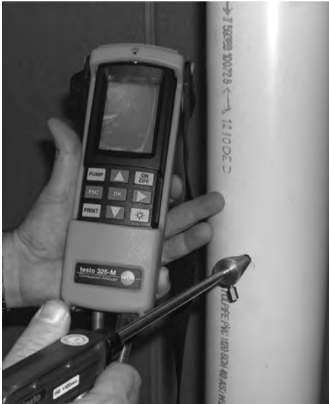
Figure 9.2: Insert Analyzer Test Probe into Test Port
