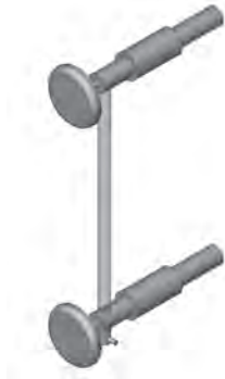
Figure 6.4: Gauge Glass Installation
