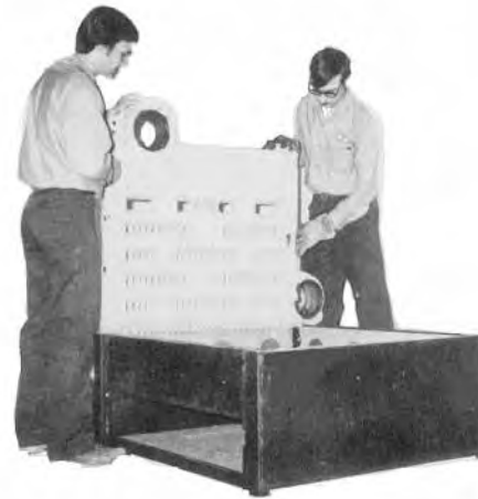
Figure 3.2: Placing the First Section on Base
