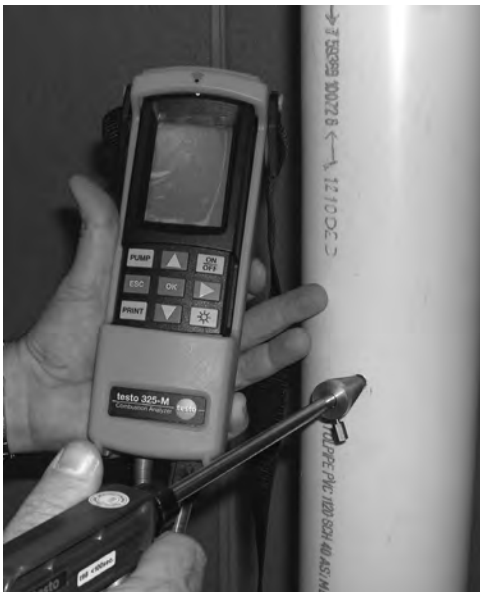
Figure 9.3: Insert Analyzer Test Probe into Test Port
