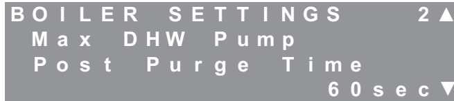
Figure 8.34: Maximum Pump Post-purge Time
