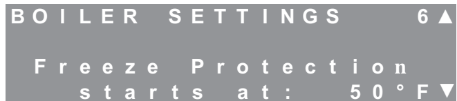
Figure 8.38: Freeze Protection Starting Temperature
