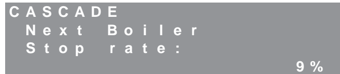
Figure 8.60: Next Boiler Stop Rate
