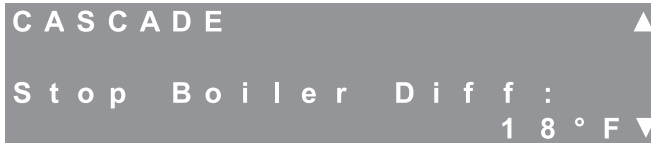
Figure 8.57: Cascade Stop Boiler Differential
