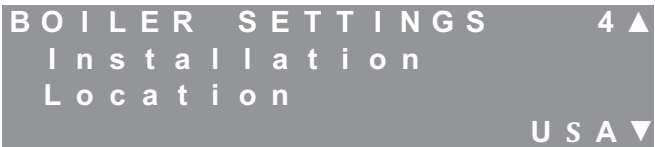
Figure 8.36: Installation Location Selection
