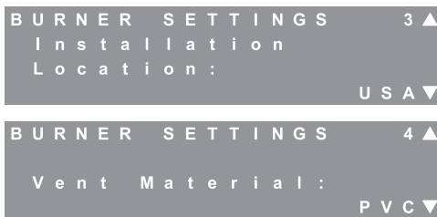
Figure 8.22: Burner Settings – Location & Vent Material
